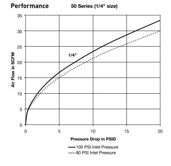
50 Series SpecificationsBody Size1/4Rated Pressure (psi)300Temperature Range (std seals)-40° to +250° FLocking Device4 ballsVacuum ServiceNot Recommended
